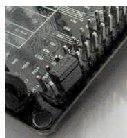
< Jumper in Boot Position
